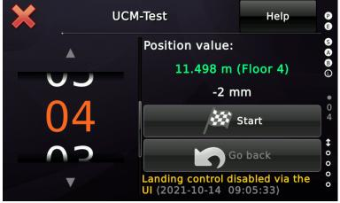
Figure 112: The main screen of the testing assistant, showing the current floor and letting the user select the direction by swiping the floor value on the left.
