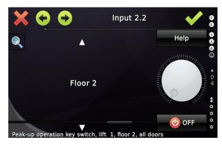
► The inputs indicating peak-up or peak-down operation have precedence over the time planner functions.
