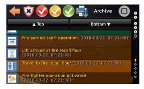
Driving to the fire recall floor and turning to 'Fire Service' operation by either using the key-switch in the car or (depending on local regulations) automatically after arrival and door opening in the fire recall floor.
