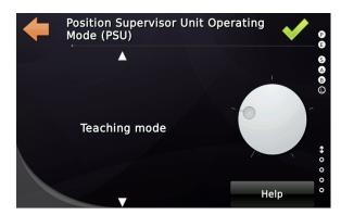
If the unit has entered '*Teaching Mode*', the PSU can be setup by entering the '*Configure & Teach*' menu.
