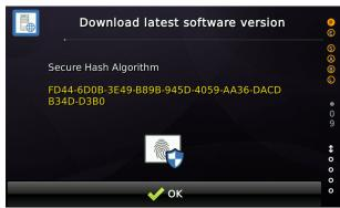
In the case the hash does not match or has been entered wrong, the update process can not be executed. Otherwise the update will be installed.
