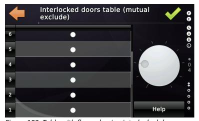
Figure 182: Table with floors, having interlocked doors.
