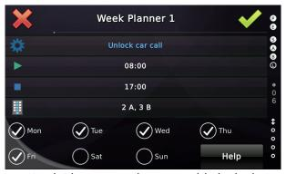
Figure 90: Week Planner used to re-enable locked car calls
