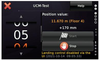
Figure 114: The test has been started going upward with the safety chain bridged by the THOR-SZ board. The stop-button may be used to cancel the process.
