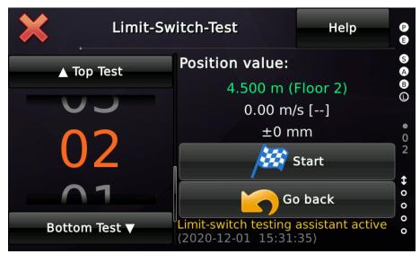
Figure 102: Driving to a floor before an end stop.
