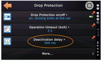
Figure 127: Defining a delay for operating the bolt after the lift has stopped
