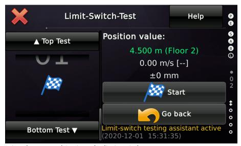
Figure 103: Starting the test to drive into the limit switch.
