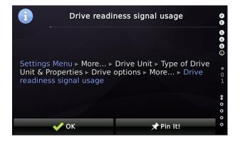
• If you have a wired overpressure indication as well, you will need to connect that one to *Drive Unit Signals* → *Hydraulic oil overpressure*, *lift 1*. In order to use that input, tell the lift controller to monitor it, by turning the corresponding option on as well:
