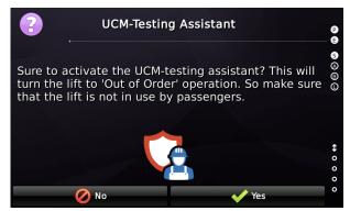
Figure 109: Security query to ensure the assistant is activated with purpose.
