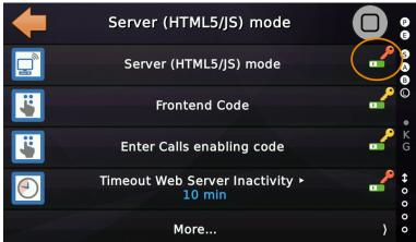
**3.)** After the set inactivity time has expired, the random Ticket Code for the display control expires and the parameterized Front-end Code must also be re-entered. To use it, all you need is a web browser on your phone. We recommend using the Opera® Mini web browser on mobile as it has a full screen mode.
