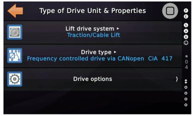
Figure 156: Type of Drive Unit Parameter
