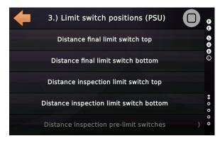
After the reference points have been taught, the teaching operation can be started by using the corresponding menu and selecting '*Learning Trip*'. The current floor level positions are erased. Before starting the learning trip, the car must be moved flush to the lowest floor level, using the inspection/emergency electrical operation.
