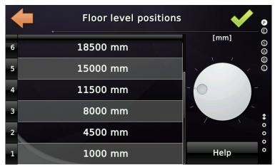
Figure 51: Adjusting the floor level positions
