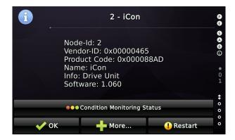
Whether there is a connection to the 'iCON CANopen' can also be checked in the node list, where the iCON should typically appear as node 2.
