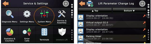
Figure 21: Lift Parameter Change Log found under System Menu → Security
