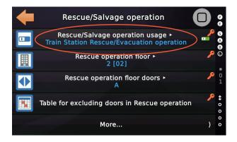
Use the 'Rescue operation floor' to define the floor where the people are driven too. Usually the ground floor, if speaking about a Train Station. Also define the door that shall open.
