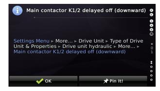
• Indicate to the lift controller, that the status information is send via the bus system, like so:
