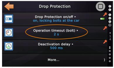
Figure 126: Option for defining the supervision time for operating the bolt
