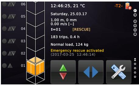
Figure: Lift being on inspection/emergency electrical operation.
