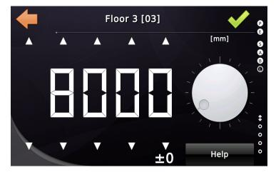
To store the changed value, tap on the green check mark button. If you have finished altering the floor level values in the 'Floor Level Position Table' tap the same button in the table too. Only then the values will be stored to non-volatile memory all in once.
