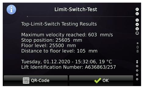
Figure 104: Test result, shown if the test was executed.
