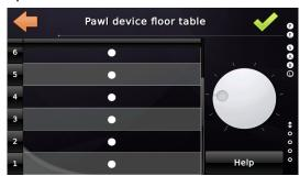
Figure 193: Table for defining the floors that feature the pawl device
