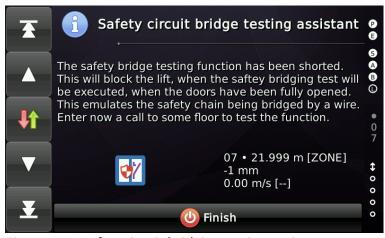
Figure 122: Safety circuit bridging testing assistant
