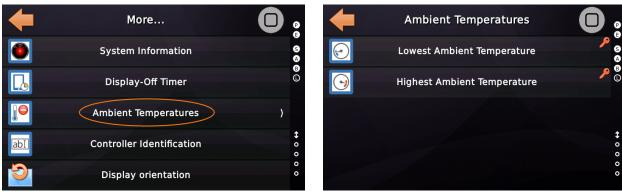
Figure 188: Lowest/highest allowed ambient temperature settings
