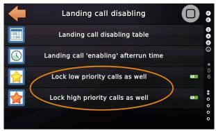
Figure 91: Locking priority calls together with landing calls
