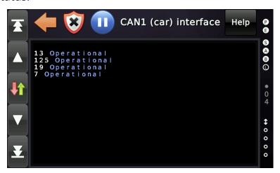
All inputs, outputs, door commands, door status words, PSU commands and PSU status words, bus errors and the status of the digital load measurement, that are then transmitted via the bus system are translated into readable text.
