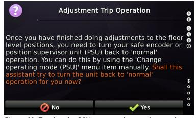
Figure 60: Turning the PSU to normal operation mode
