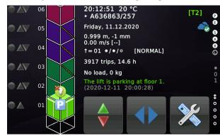
Figure 93: Hoistway divided into zones
