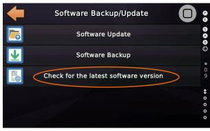
For downloading an update file via the cloud service, you want to choose 'Check for the latest software version'. If the connection with the cloud is successful, you will see the current installed version and the version that can be downloaded as an update.
