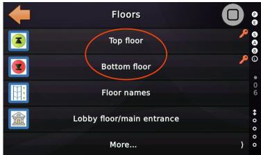
Figure 26: Top/Bottom Floor Level Settings
