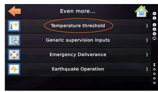
The temperature threshold outputs will be turned on, if the temperature exceeds the given value. In the example, the virtual output for the '*Temperature threshold 1*' will be turned on, if the on-board temperature sensor detects an ambient temperature over 38 degree Celsius.
