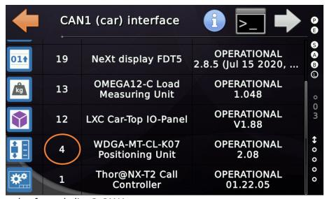
Figure 25: Example of a node-list @ CAN1
