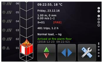
Figure 138: Lift in Fire-Alarm-Operation mode.
