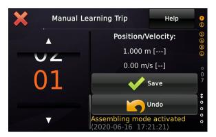
Move the car now by operating the lift via the inspection/emergency electrical operation panel up and down to the next floor level. If you have a second person to support you, it might be easier. Otherwise you can monitor the state of the door zone magnet switch.
