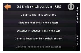
After the reference points have been taught, the teaching trip operation can be started by using the corresponding menu and selecting 'Learning Trip'. The current floor level positions are erased. Before starting the learning trip, the car must be moved flush to the lowest floor level, using the inspection/emergency electrical operation.
