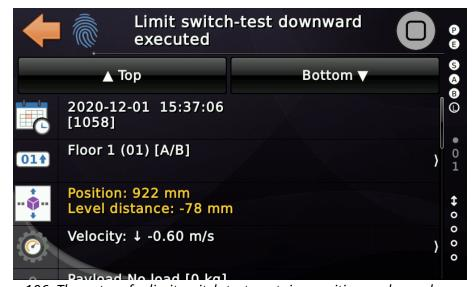
Figure 106: The entry of a limit switch test contains position and speed
