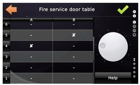
Figure 147: Fire service cross-out door table
