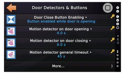
Figure 179: Door Detectors & Buttons
