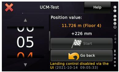
Figure 119: Touch the 'Go back' button to start driving back to the floor.
