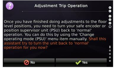
Figure 52: Turning the PSU to normal operation mode
