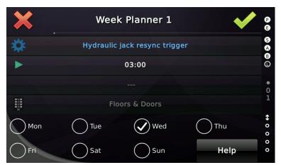
Figure 197: Time Planner used to trigger the hydraulic jack resync
