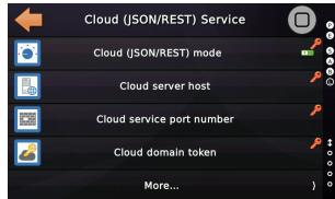
The connection parameter, such as the host name and the port number, as well as the domain token, shall be obtained from your cloud provider.
