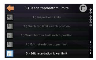
As soon as the limit switches and retardation positions have been taught, the learning trip can be started. To do so, change to the corresponding menu and select the learning trip. The current floor level positions are deleted. Before starting the learning trip, the car must be moved flush to the lowest floor, using the inspection/emergency electrical operation control. This is the starting point for the learning trip. Afterwards, the assistant is opened for the manual learning trip operation.
