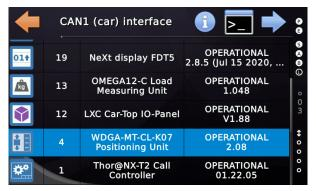
Figure 152: CANopen Node List, showing the encoder
