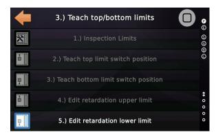
As soon as the limit switches and retardation positions have been taught, the learning trip can be started. To do so, change to the corresponding menu and select the learning trip. The current floor level positions are deleted.
