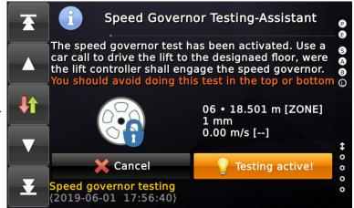
the testing results, containing the maximum velocity reached and the distance that it had taken from engaging the bolt to stopping the car.
