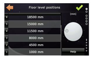
After the learning trip has been finished, it is now possible to drive the lift using nominal velocity. Before continuing with the 'Adjustment Trip' in the next step, the floor level positions, braking distances, drive parameters can be optimized until the lift stops flush on every floor.
