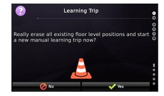
Figure 28: Erasing all existing floor levels
