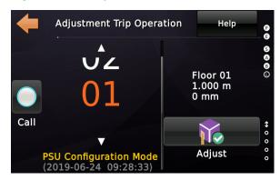
Using the call button on the left, the lift will start to drive to the selected floor. As soon as the lift arrives at the floor, the position can be transmitted to the PSU via the 'Adjust' button.
