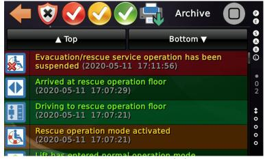
Figure 146: Evacuation operation suspended via an input signal
