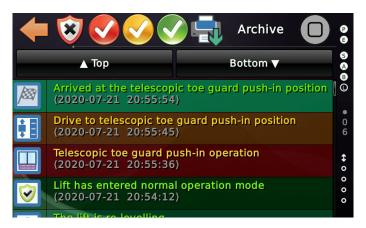
In the event of an error, the procedure is finished with the information that the telescopic toe guard could not be pushed-in again. The lift will then remain 'out of order' on the bottom floor. Usually the car is brought back to the lowest floor level position by a re-levelling operation.
