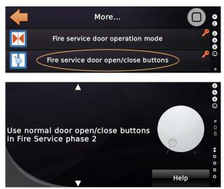
If you feature special door open/close buttons, just for a Fire Fighter panel, use the 'Door Controlling Signals  $\rightarrow$  Fire service door open/close button, lift 1, car/cabin, door X' for that purpose. For the signal lamps, indicating that the fire fighter can operate the open/close buttons, use the 'Door Controlling Signals  $\rightarrow$  Fire service door open/close button acknowledge, lift 1, car/cabin, door X'.
