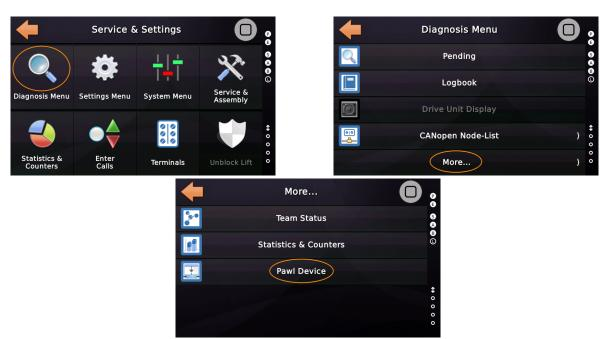
Figure 194: Path to the pawl device status
