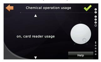
The input function 'Status/controller signals  $\rightarrow$  Chemical transport' indicating the floor and door side where the card reader is located is used for this variant. The input function 'Status/controller signals  $\rightarrow$  Chemical transport reset' remains available and could also be used in this variant if required or desired.
