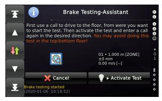
Then the technician may active the test via the the 'Activate Test' button. If several brake circuits had been parameterized, the software will now ask for the brake circuit, that shall be tested. If just one brake circuit had been parameterized, entering the brake number is not necessary.
