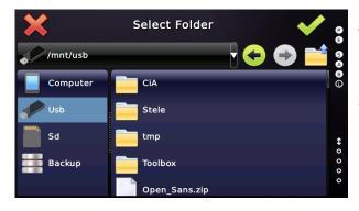
Touching the green check mark symbol will now store the printout to the USB mass storage. You will find the events, the help texts and the counter values included in the printout. The text file is UTF8 (Unicode) encoded and shall therefore be fine for usage on any up-to-date system.
