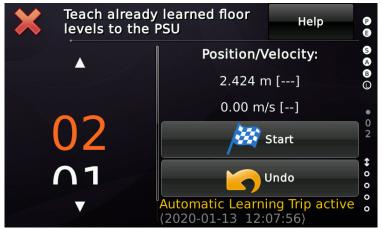
Figure 46: Automatic Adjustment Trip Assistant
